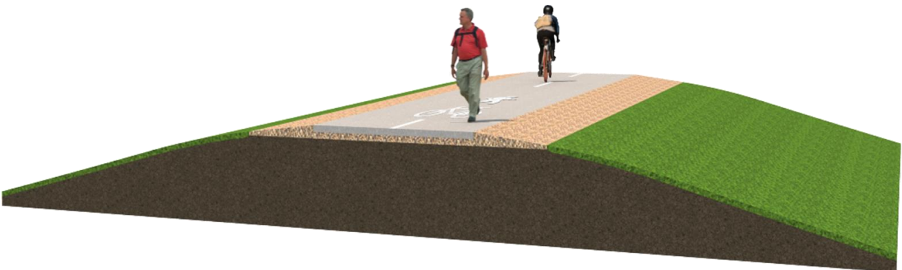
3D Concept Drawing – typical cross section – 2.5 metre wide concrete shared path on existing levee bank formation
