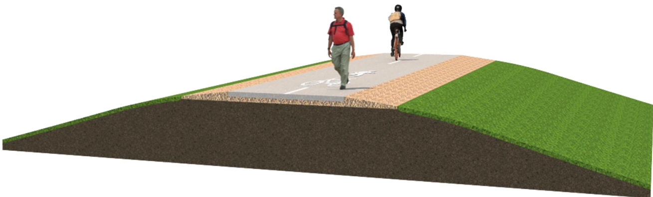
3D Concept Drawing – typical cross section – 2.5m wide concrete shared path on existing levee bank formation
