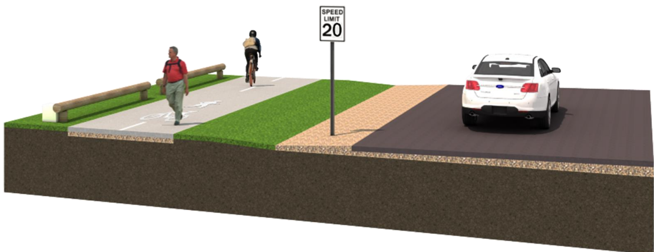
3D Concept Drawing – typical cross section – new 2.5m wide concrete shared path and shared path signage
