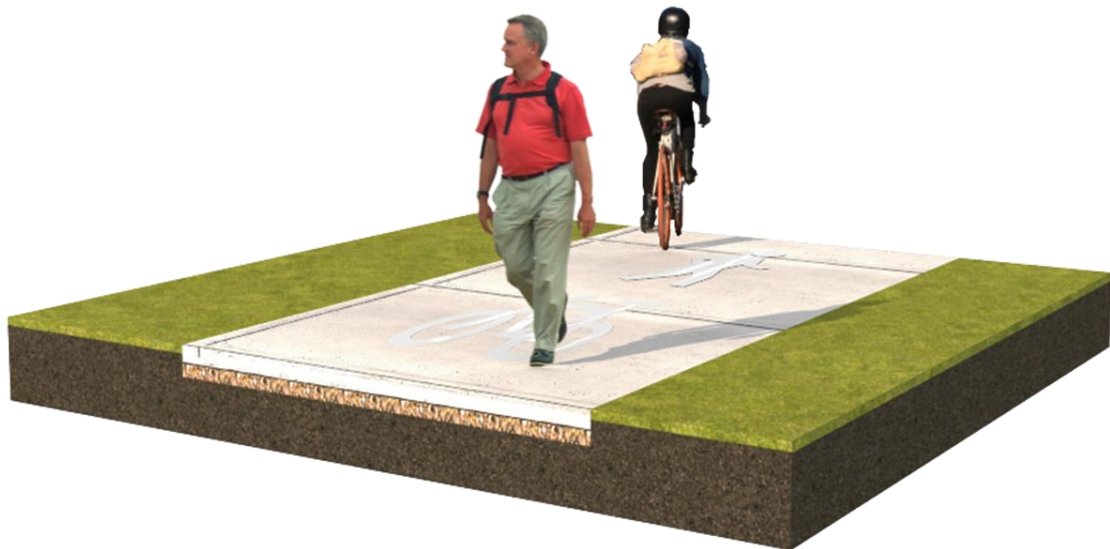
3D Concept Drawing – typical cross section – 2.5m wide concrete shared path
