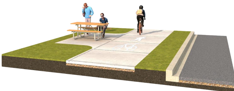
3D Concept Drawing – typical cross section – 2.5m wide concrete shared path with rest seating installation
