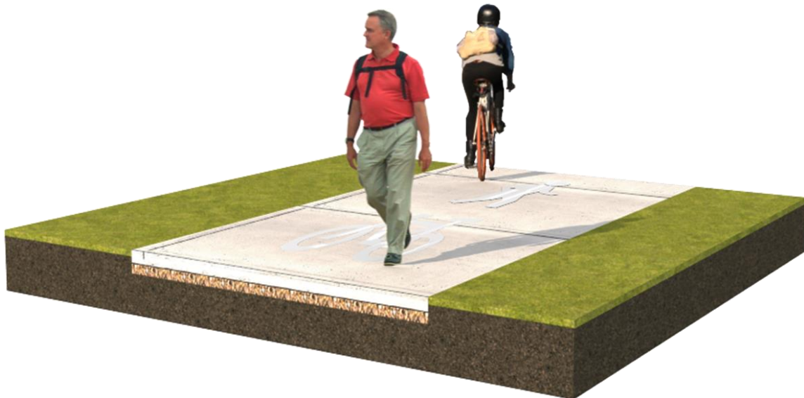
3D Concept Drawing – typical cross section – 2.5 metre wide concrete shared path
