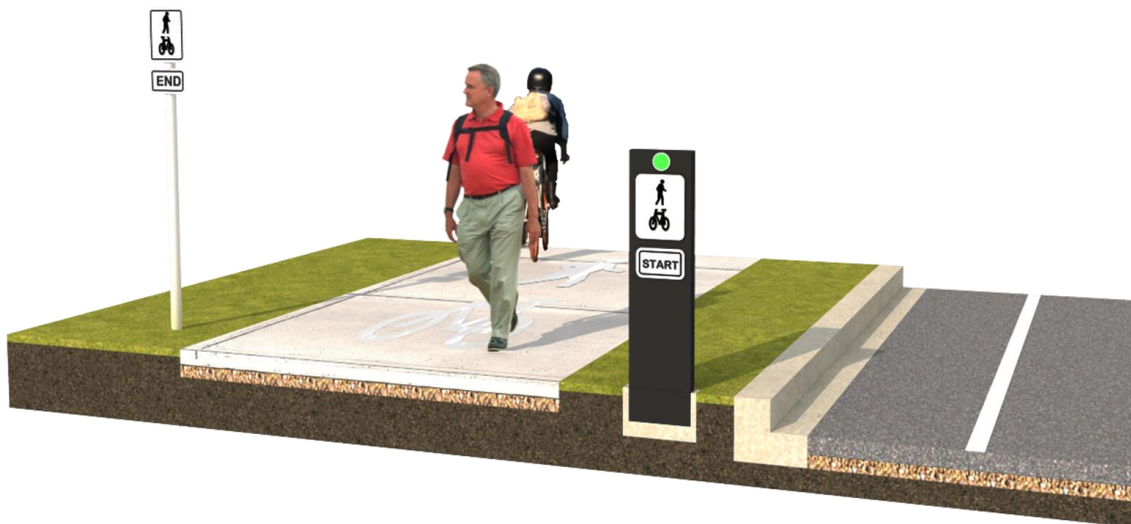
3D Concept Drawing – typical cross section – new 2.5m wide concrete shared path and signage examples
