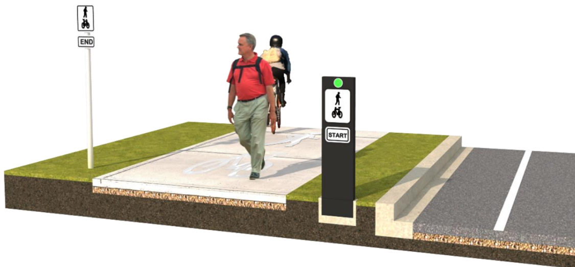
3D Concept Drawing – typical cross section – 2.5m wide concrete shared path and signage examples.
