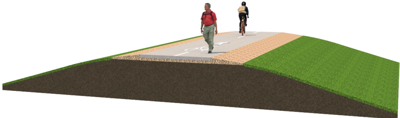
3D Concept Drawing – typical cross section – new 2.5m wide concrete shared path on existing levee bank formation
