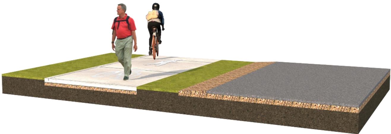
3D concept drawing – typical cross section – 2.5m wide concrete shared path
