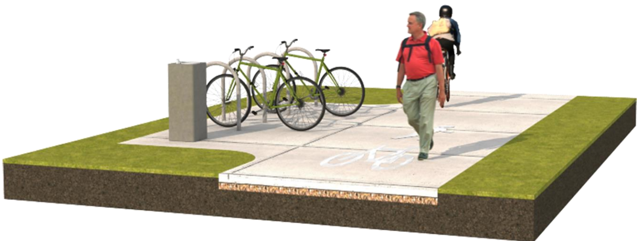
3D Concept Drawing – typical cross section – bike rack and water point installation
